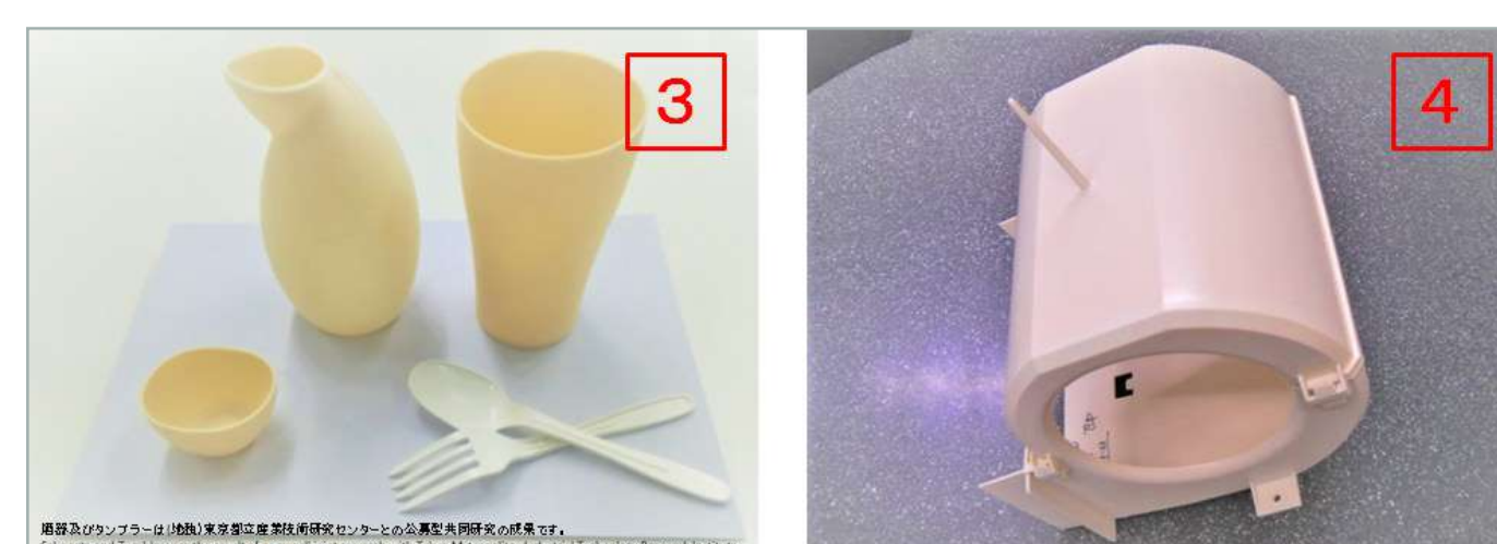
図3 生分解MAPKA(射出成形・ブロー成形)と カトラリー(射出成形) Fig.3 Paper powder and PLA, PBS (Injection molding / blow molding) Spoon and Fork(Injection molding)
